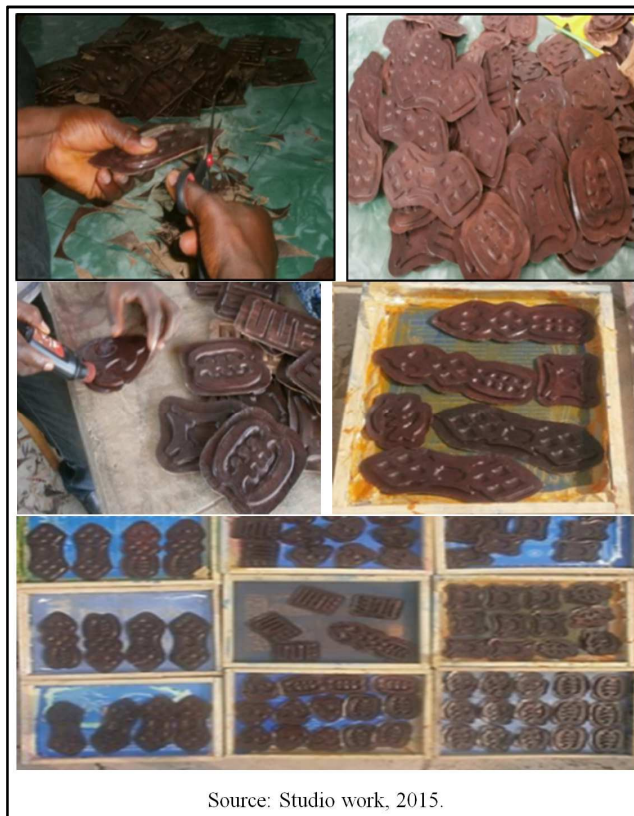
Figure 16. Finishing of the moulded leather.
