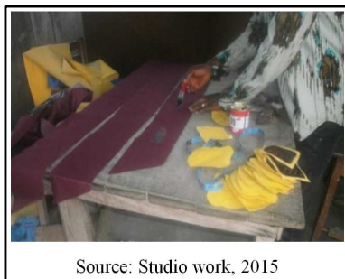
Figure 29. Fixing patterns on straps for stitching.
