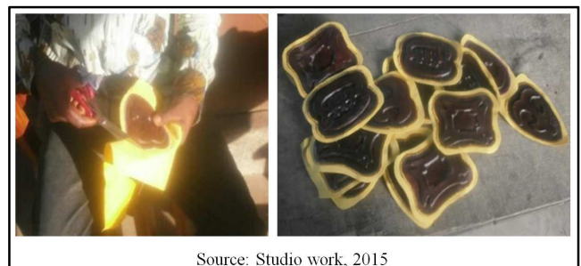
Figure 27. Trimming of backing fabric of moulded leather patterns.
