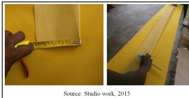
Figure 17. Measuring, cutting and folding fabric for the blind.
