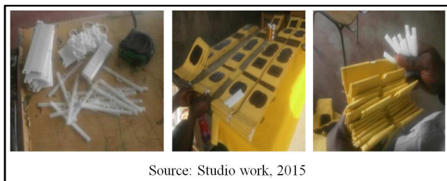
Figure 23. Blind accessories being fixed in the straps.
