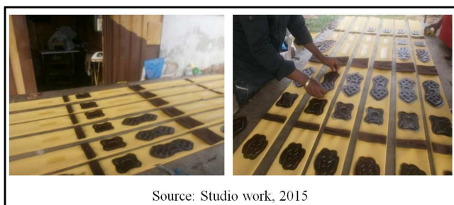
Figure 18. Arranging and fixing moulded leather on fabric for easy stitching.
